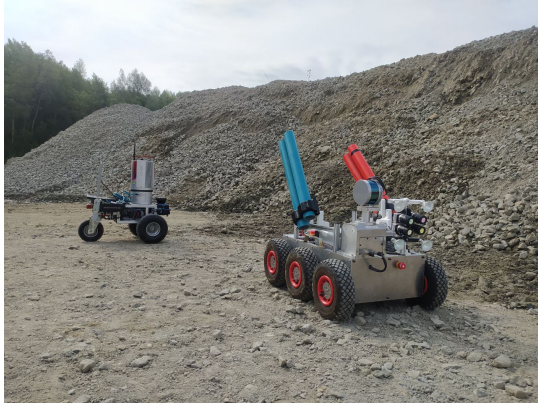
Fig. 2: The robots that the astronauts will control: Robot “Lars” (left) with a laser scanner and “Charlie” (right) with four monochrome cameras for rock analysis and the sensor distribution system to launch UWB sensors.
